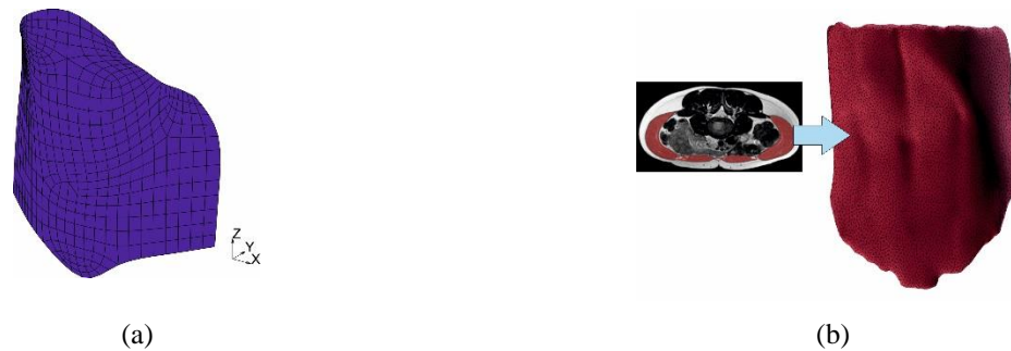
FIGURE 1. Considered models (a) membrane model, (b) solid model created on the basis of MRI images
